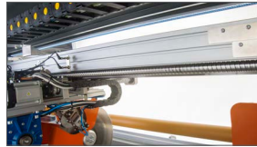
X and Y axis controlled by brushless motor system
