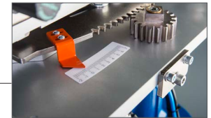
Adjustable blade angle
