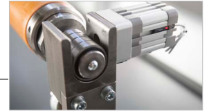
Pneumatic lifting and lowering of the mandrel to facilitate the loading and unloading of the log rolls and slit reels
