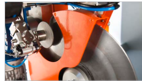
Adjustable blade sharpeners
