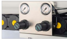
Adjustable sharpeners pressure
