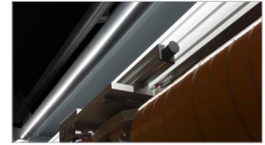
LED illumination in cutting area
